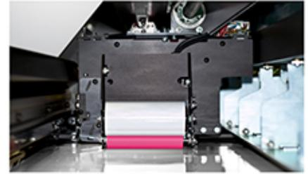
The OptiPrint™ Media Pre-Cleaning System is a unique process which removes dust and debris from the media surface prior to printing, ensuring optimal conditions for pristine quality graphics.
